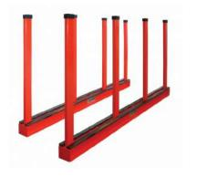
Rack is designed to store bundles of marble and granite in your warehouse or slab yard. The Bundle Rack has a Total Weight Capacity between Poles of 24,000lbs (11,000kg). Each pole is 2" x 4" x 1/4" x 59" (50 x 100 x 6 x 1500mm), and each steel rail base is covered with an additional strip of wood to protect the slabs from chips and scratches.
