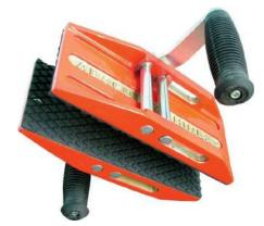
Abaco Double Handed Carry Clamps are designed to safely lift and transport stone slab without using a forklift truck. The fully vulcanized rubber pads provide added grip and prevent from damage to the slab. The weight of the slab exerts a sufficient clamping force for such a simple lifting device. By eliminating the use of a forklift truck, the Carry Clamps help users to work more efficiently works. You can use multiple Carry Clamps to move larger slab with ease.
